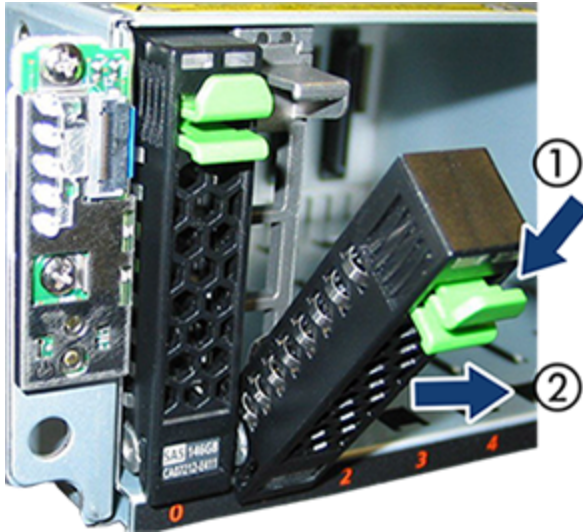
Figure 63: Removing/Installing hard disk drive
